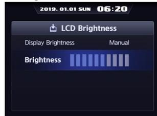
Brightness can be changed using Up/Down button when it is manual mode.
