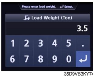
Enter load weight using up/down buttons.
