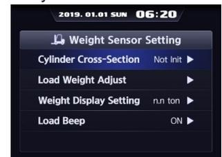
Choose Cylinder Cross-Section. If Cylinder Cross-Section is already set up, setting value is shown in initial screen.
